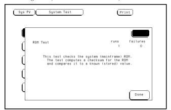
For a Single run, the test runs one time, and the screen shows the results.
